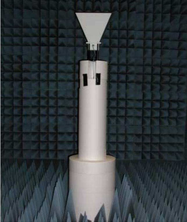
Figure 10. DUT Fixtured on Foam Pylon
