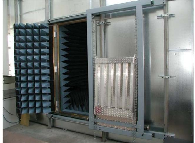
Figure 6. 5m Chamber DUT Access Catwalk
