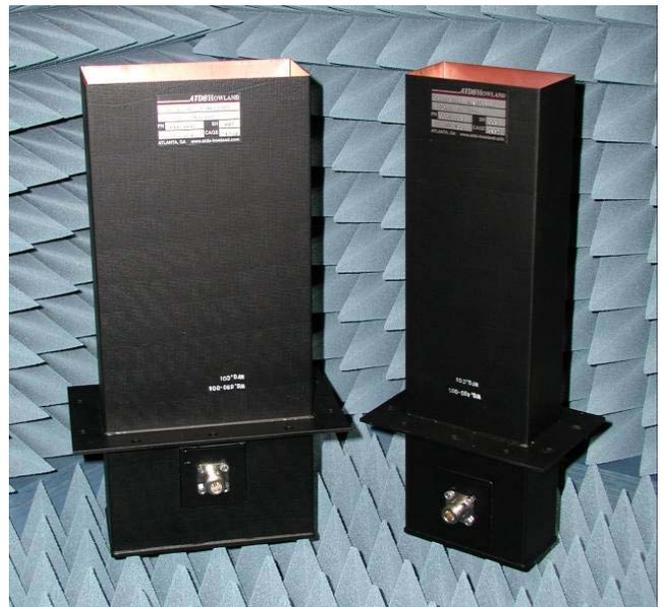
Figure 7. Low Mass OEWG Probe Antennas
