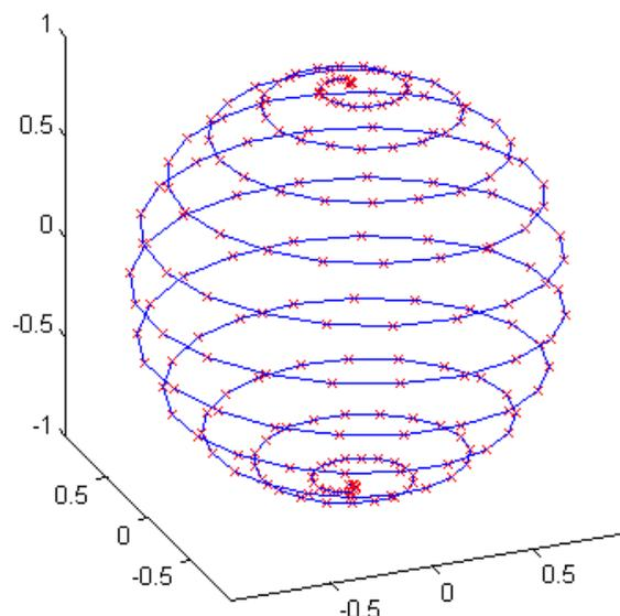
**Figure 1, Spiral scanning path. Data are collected at the marks along the path.**
