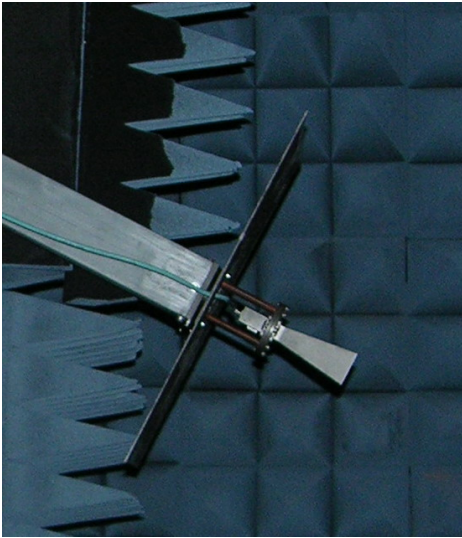
Figure 4. Spherical Probe Antenna Assembly
