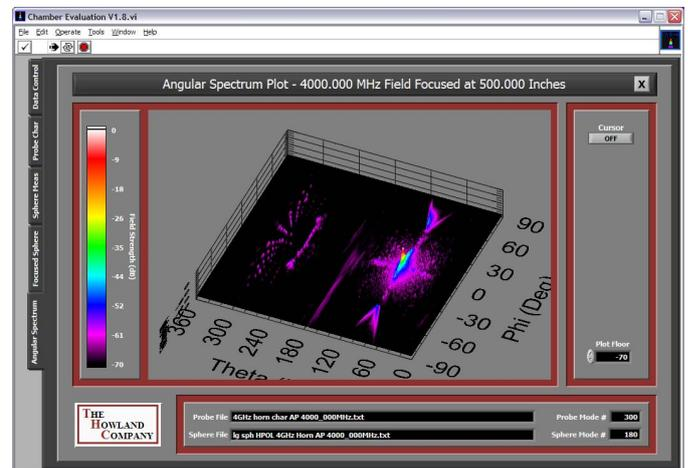
Figure 8. Angular Spectrum for Large Chamber at 4 GHz.
