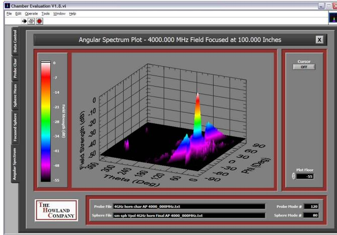
Figure 5. Angular Spectrum for Small Chamber at 4 GHz.
