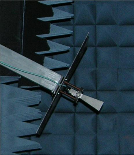
Figure 4. Spherical Probe Antenna Assembly
